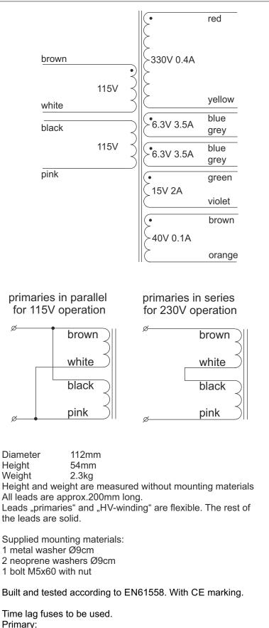
For 115V mains: 2A 5x20mm IEC127 high l<sup>2</sup>t-value in series For 230V mains: 1A 5x20mm IEC127 high l<sup>2</sup>t-value.
